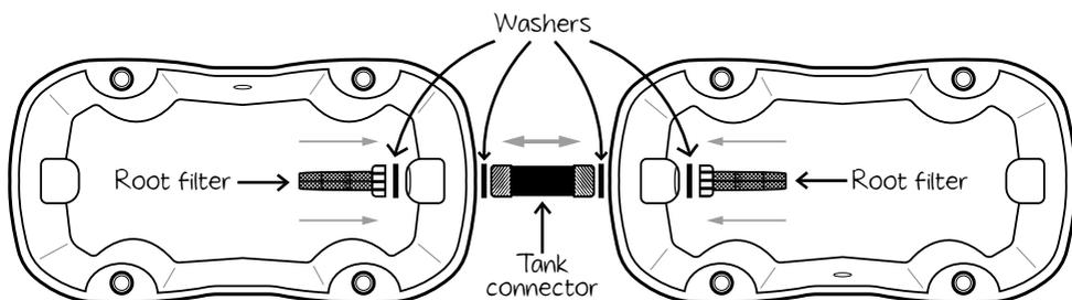
5. Use the spanner to tighten the Root Filters onto the Tank Connector on the inside of each SmartReservoir (see image).
